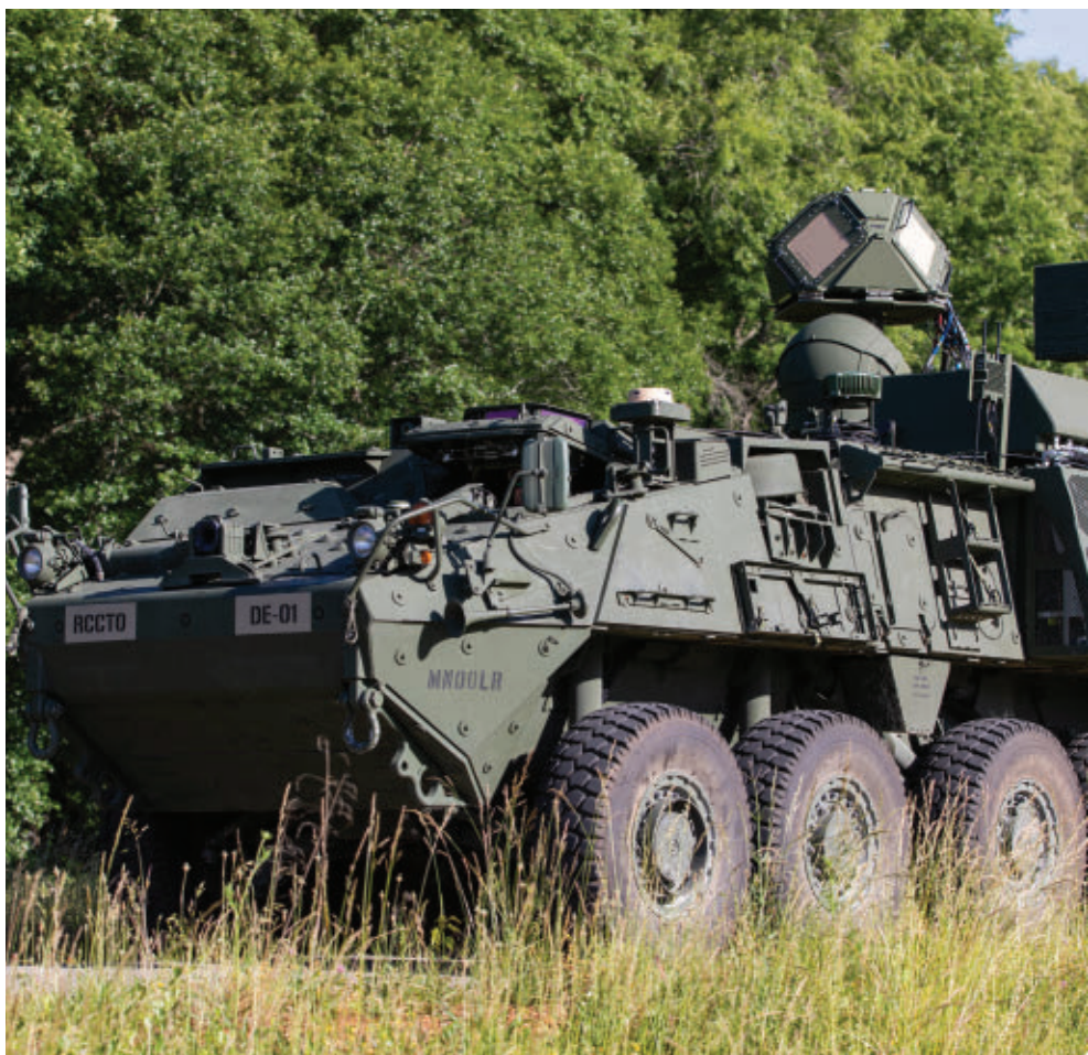
DE M-SHORAD 50-kilowatt mobile air defense laser weapon can shoot down manned and unmanned fixed-wing aircraft, helicopters, and missiles.
